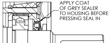
PULLEY END DETAIL
