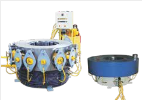
◀ 600 tons High-Accuracy Collar Press. For the production of accelerator coils, sheet metal needs to be formed into a specific shape and size.
