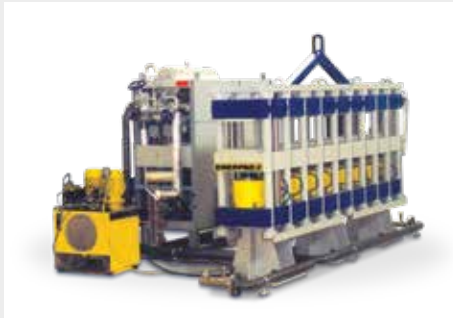
◀ Fully Automated PLC-Controlled 1800 tons, High-Accuracy Press. The pressing and heating cycle, during the production of magnetic acceleration coils, required high force and high- accuracy to ensure absolute quality
