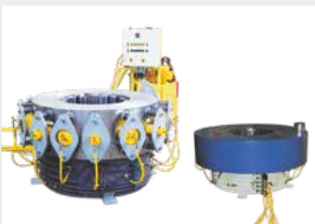
◀ 600 Ton High-Accuracy Collar Press. For the production of accelerator coils, sheet metal needs to be formed into a specific shape and size.
