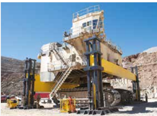
◀ A 1200 ton electric mining shovel being separated using custom 500 ton RR-Series cylinders and a pump per point synchronous lift system.
