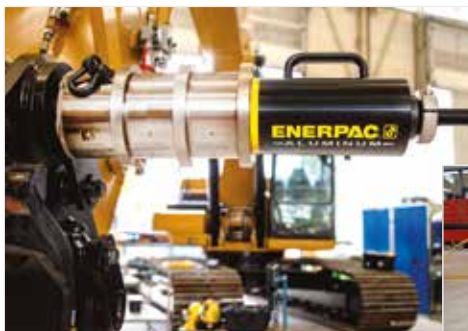
◀ Excavator maintenance using the PPH40 powered by a SC-Series Cordless Pump.
