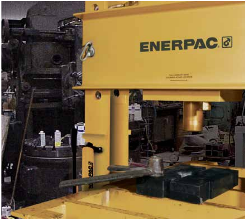
▲ An IPR20075 Roll Frame Press is used to remove a large shaft from this pillow-block assembly. The Roll Frame design allows this heavy part to be safely loaded with an overhead crane.
