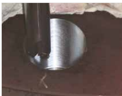
▲ New machined thread.
