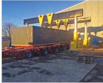
Hydraulic boom gantry safely transports 120 tons machine bed.
