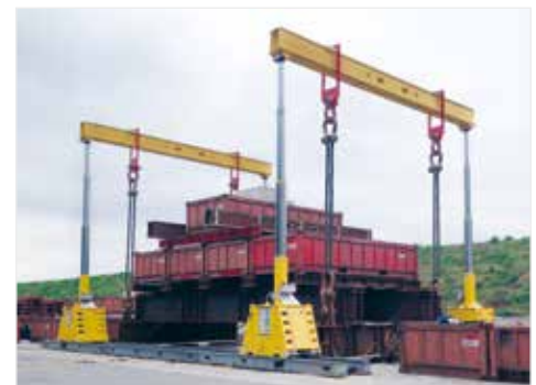
SL400 Gantry during load testing. ►
