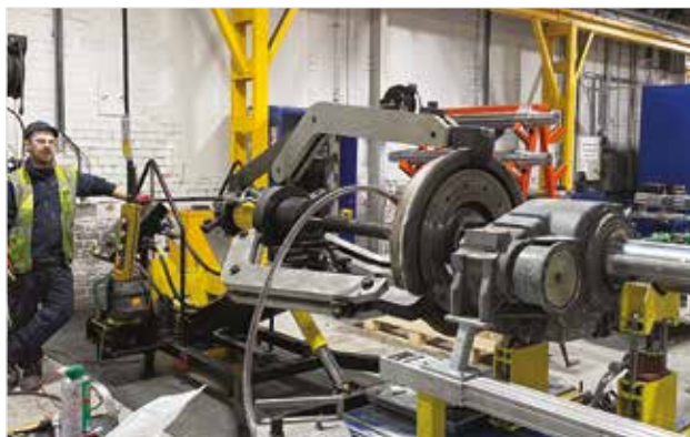
◀ LGH3100 used to remove rail wheel from axle.
