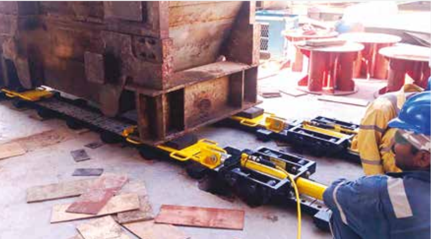
Low-Height Skidding System provides the ability to maneuver and transport large, heavy objects like this press frame.
