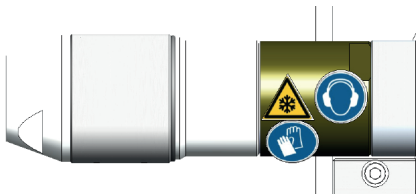
Figure 2: Motor showing safety labels
