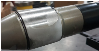
Figure 3: Frost/ ice on Motor
