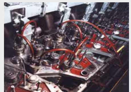
▲ Hydraulic nuts on a diesel engine.
