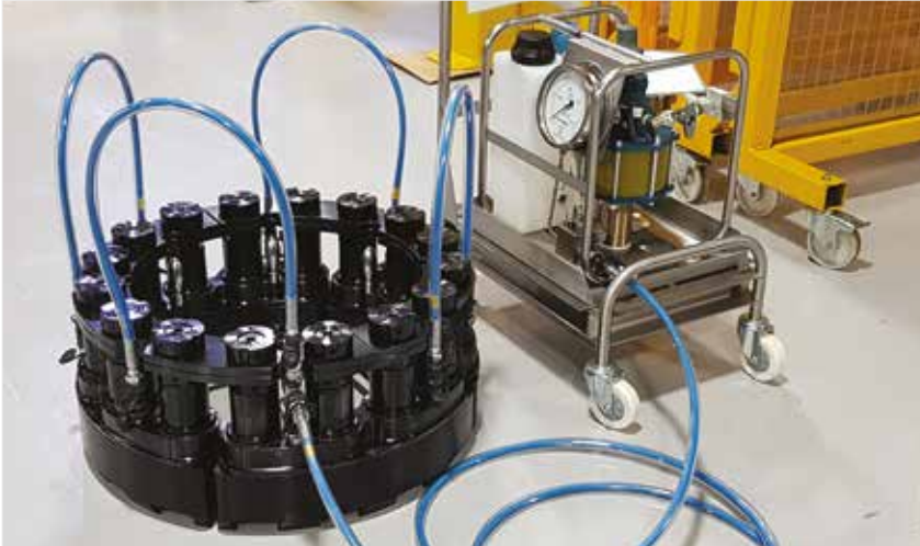
▲ Multi Stud Tensioning Set-Up.
