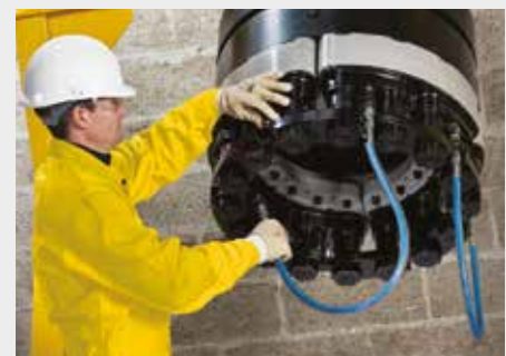
▲ Multi Stud Tensioning application.
