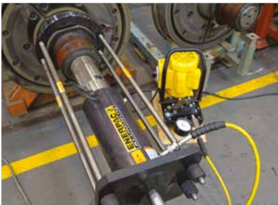
◀ Rail wheel pulling using RACH-aluminium cylinder powered by ZE-Series pump.
