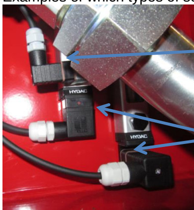
Seals of oil temperature switch
