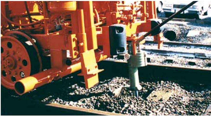
▲ Model TJ109S is shown lifting a rail maintenance car.
