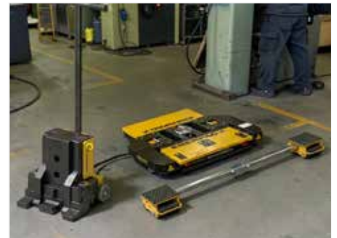
▼ Machine lifting with Toe Jack and horizontal movement using EMLS-Series Battery-Powered Machine Skates.
