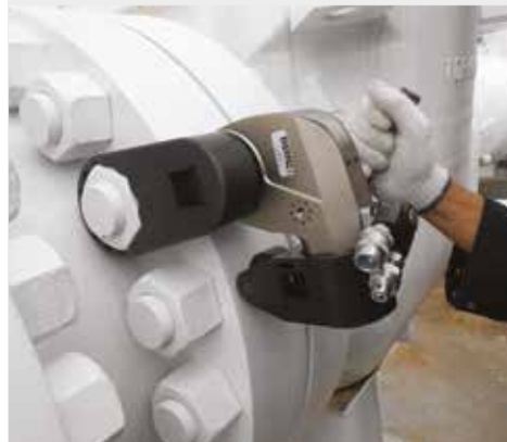
▲ Custom S11000X torque wrench with a custom torque link and reaction roller.
